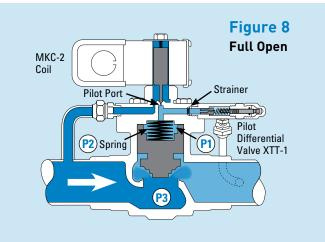
the main piston. These valves are available in two port sizes, the (O)LDR-16 (1") and the (O)LDR-20 (1-5/16"). Inlet pressure enters the pilot assembly through a passageway in the valve body on the (O)LDR-16, and through an external tube connected to the inlet fitting on the (O)LDR-20. The outlet on the pilot differential is through an internal passage in the valve body on the (O)LDR-16, and on the (O)LDR-20, the valve is connected to the outlet fitting with an external tube.
