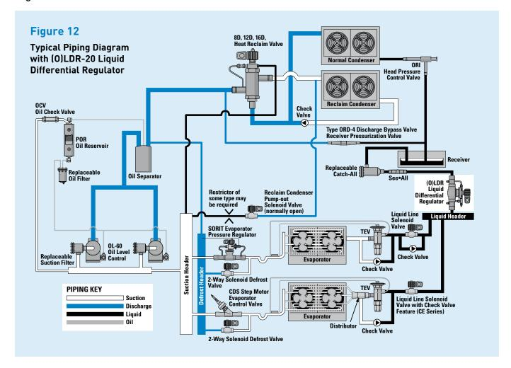
A normally open OLDR version or an LDR version (differential mode when the coil is de-energized) must be determined if a liquid differential pressure regulating valve is desired.
