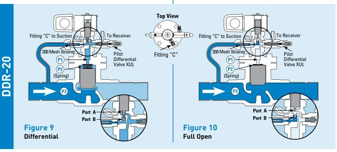
a greater pressure than the liquid header. Correct application depends on several factors. Either of the two types of defrost differential pressure regulating valves (liquid line or discharge line) can be applied on supermarket systems. However, the two types cannot be applied on the same system. Latent gas defrost requires the differential valve be in the liquid line.
